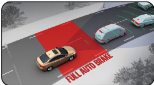
Collision Warning with full autobrake Active between 4 - 200 km/h
