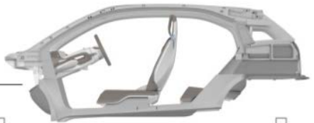
Life-Modul with CFRP passenger compartment
